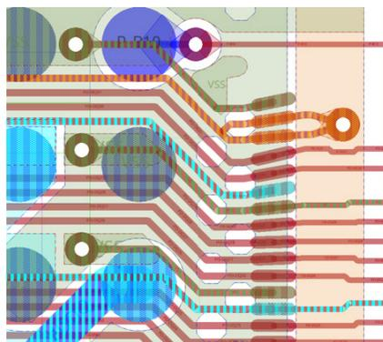
Figure 5: Constraint-driven interactive, auto-interactive, and full auto-routing tools are included that support orthogonal, 45s, and any-angle routing.
