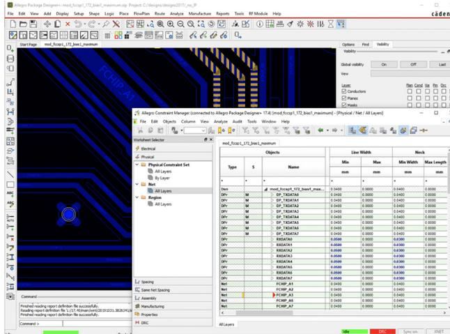
cations for critical nets. DesignTrue DFM checks ensure designs meet manufacturers' requirements. Designs can be dynamically checked against these constraints throughout the design process to ensure they are meeting manufacturing and electrical specifications. Immediate feedback is provided by DRC markers as well as flagging violations in the spreadsheet-based Constraint Manager.
