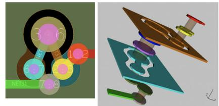
Figure 6: Constraint-driven HDI design allows designers to rapidly implement and update repetitive complex via structures, including return path vias, for escape and layer transitions.
