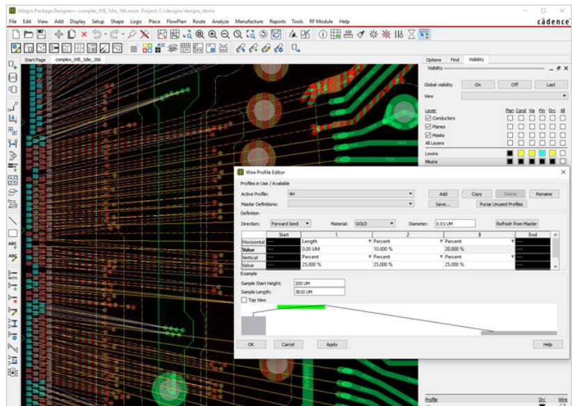
Figure 1: Constraint-driven interactive wire bonding includes push-shove across multiple wire tiers. A 3D wire profile viewer/editor allows for multiple wire profiles to be created and supported. Referenced profile libraries enable manufacturing-aware design and accurate simulation.
