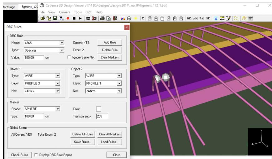
Figure 8: 3D interference rules (wire to wire and wire to object) are available through the 3D Viewer (included), using accurate wire curvature models.
