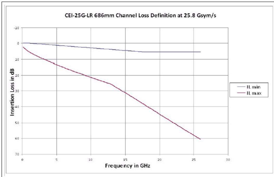
Figure 11-2. CEI-25G-LR Normative Channel Insertion Loss at 25.80 Gsym/s.
